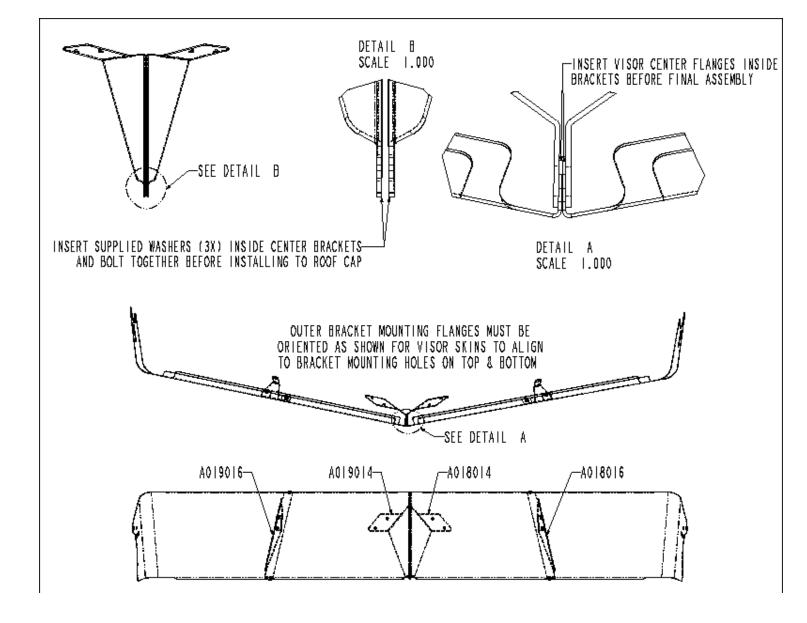
**Note:** The brackets for the Sunvisor must be installed onto the cab of the truck with 3/16" huck bolts to insure a secure and watertight installation. It is recommended to have the brackets installed at a factory authorized repair center. The fasteners included with this Sunvisor are intended for attaching the Sunvisor to the brackets
