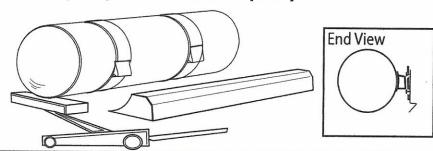
Step 2 A) With brackets on the tank, hold the Fairing in position and mark where the brackets are located on the Fairing.
