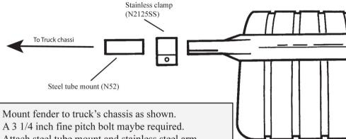
A 3 1/4 inch fine pitch bolt maybe required. Attach steel tube mount and stainless steel arm together with the provided stainless clamp (N2125SS)
