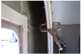
Temporarily clamp fiberglass day cab unit to factory aluminum boot ring to secure for drilling.
