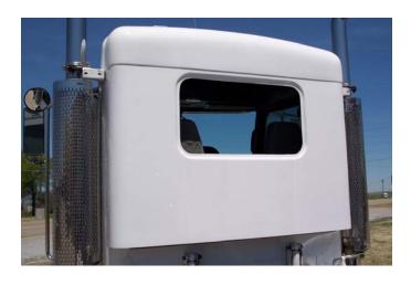
4. Fit day cab extension to cab, making certain in is centered side to side and top is flush with cab.
