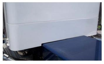
10. With air bags deflated fit lower skirt to cab, trimming may be required to allow min. ¼" clearance between frame and skirt. Bolt skirt from underside into rev-nuts using ¼"-20 bolts supplied.
