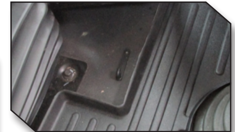
Figure 8 - Properly Installed Retention Hook
