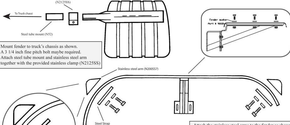
Attach the stainless steel arms to the fender as shown. Use the provided template for drilling holes. Attach bolts with steel straps on the inside of fender.
