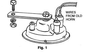
make sure that there is a 10-amp fuse used in the horn circuit to protect the vehicle. If the wire terminals that were connected to your vehicle's factory horn doesn't not connect to your new Wolo horn, provided in the kit is two (2) 1/4" push-on insulated terminals. The installation is complete and the horn is ready to be used.
