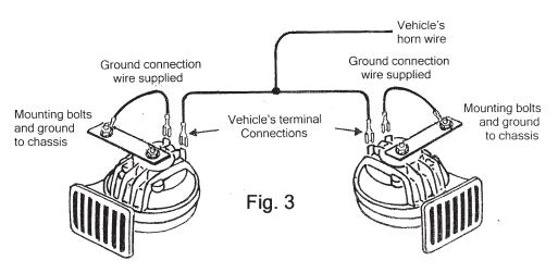
bolts of the horn and firmly tighten. Make sure the horn's mounting bracket is secured to a metal body surface that is clean of paint and rust.
